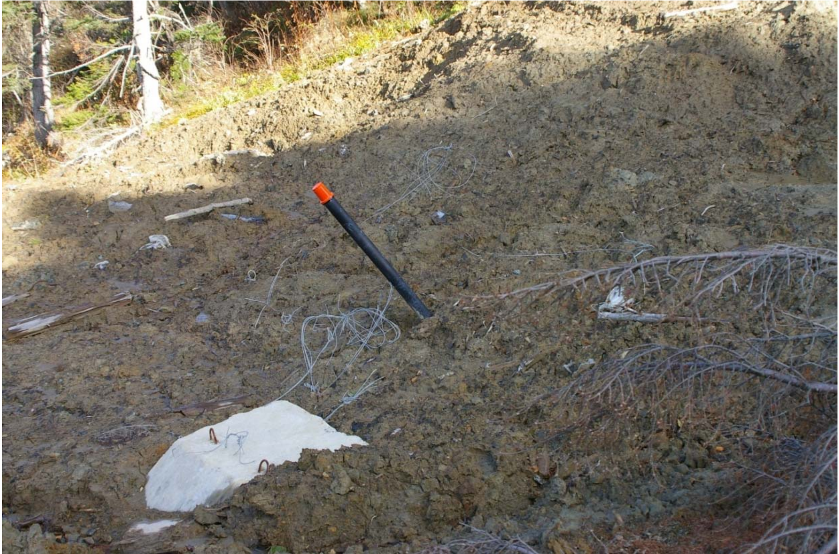
October 23, 2007: KP 482.5. The right bank of the Primorskaya River. The cathode protection check point for the oil line has been broken by the creeping land slide.
